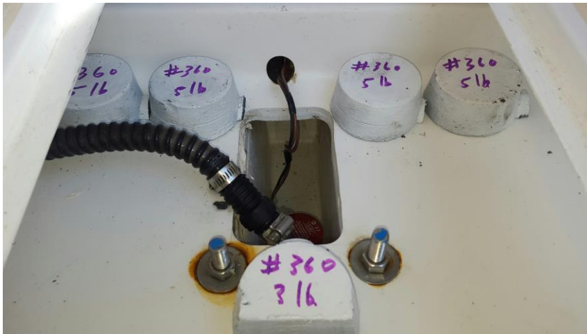
Middle Bilge at bilge pump originally to be in well aft of barney post but approved by warren Duncan to be relocated.
