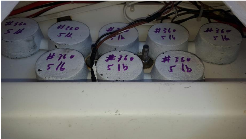
40 lbs forward bilge aft of bulk head
